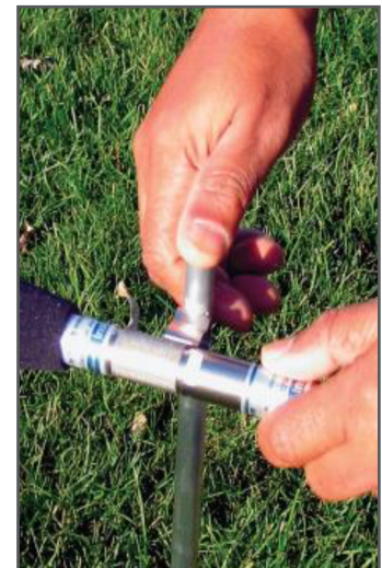
Figure 4. Installing the Microphone
