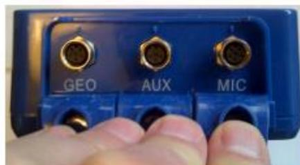
**Micromate with Auxiliary I/O installed**
