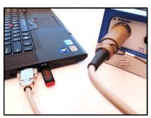
2a. Serial Cable (Part # 720A3401) to Serial port
