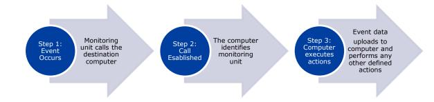
Step 1. The unit's configuration defines how communications are established when calling a computer.
