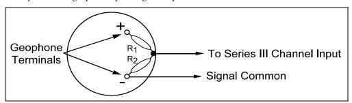
Figure 4-3 Adapting the 14 Hz Geophone.
