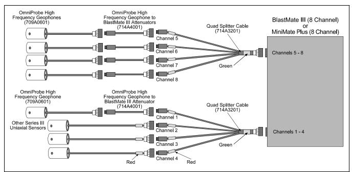
Figure 3–4 Connecting OmniProbe High Frequency Geophones and other Uniaxial Sensors to 8 Channel Monitors.
