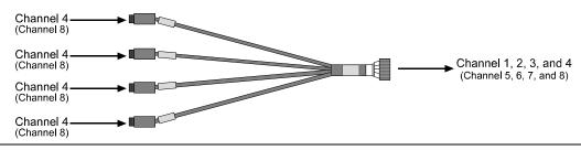
Omni Probe High Frequency Geophone to BlastMate III Attenuator (714A4001) – must be attached to the Omni Probe High Frequency Geophone in all connections.
