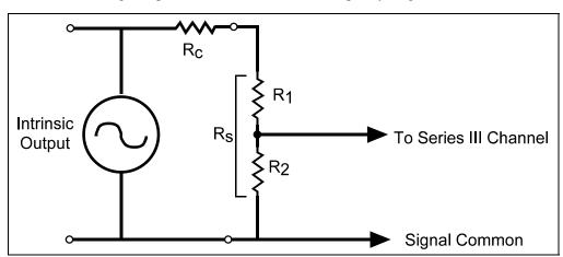
Figure 4-2 Geophone Schematic.
