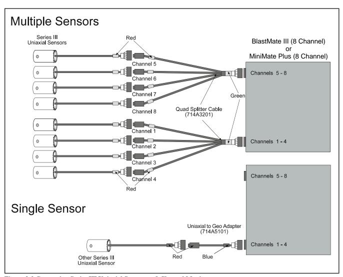
Figure 3-2 Connecting Series III Uniaxial Sensors to 8 Channel Monitors.
