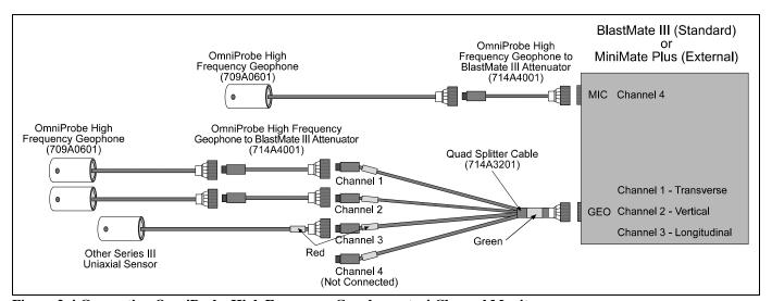
Figure 2-4 Connecting OmniProbe High Frequency Geophones to 4 Channel Monitors.
