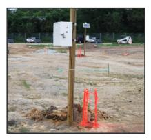
6. Borehole geophone location clearly marked with monitoring unit placed in a secure lock box.
