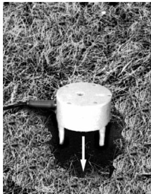
Installing the Standard Ground Spikes.
