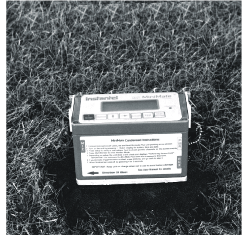
Figure 3-3 Final Installation with Ground Spikes Pushed Fully into the Ground.
