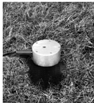
Final Installation with Transducer using the Ground Spikes Pushed Fully into the Ground.
