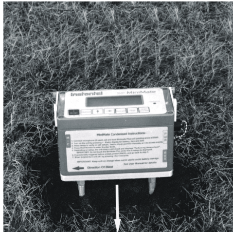
Figure 3-2 Installing the Minimate using the Ground Spikes.
