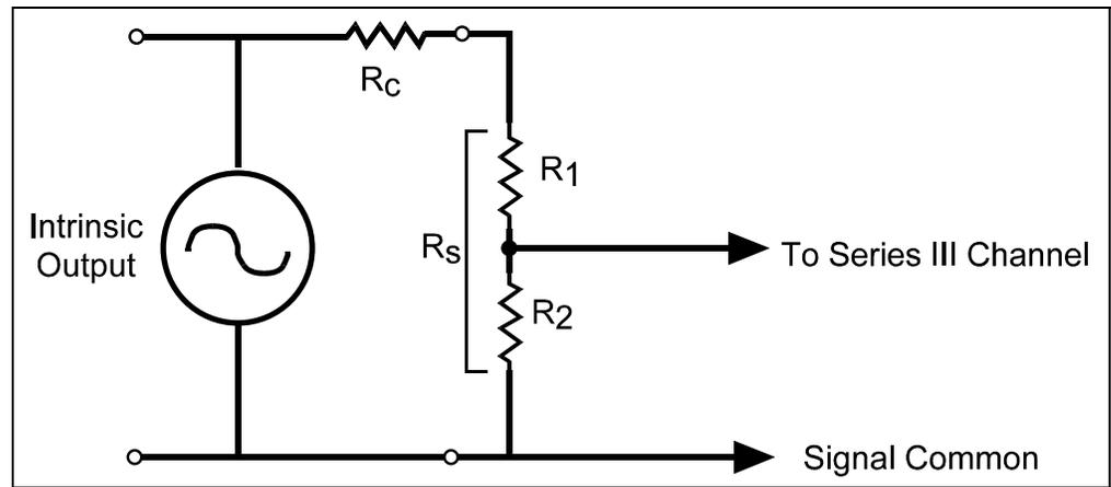
Figure 4-2 Geophone Schematic.
